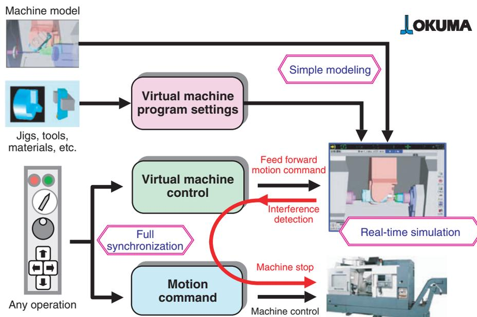
Fig. 5 Conceptual diagram of anti-crush system (Okuma Co.)
