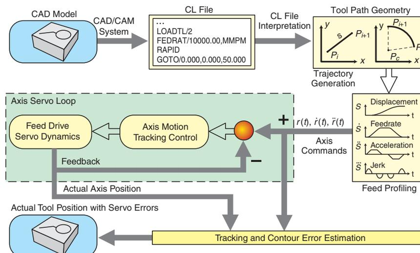
Fig. 6 System architecture of virtual CNC <sup>4)</sup>
