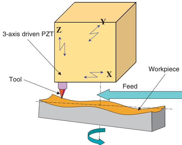
Fig. 4 Schematic illustration of ultraprecision cutting by 3-axis FTS
